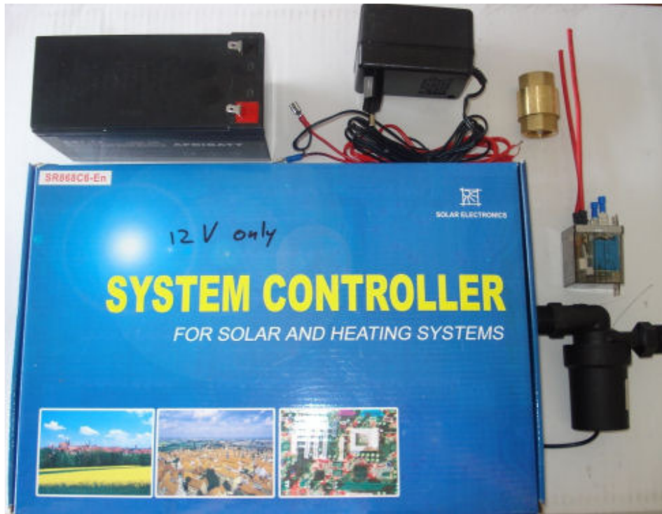
Fig 1. 12V pump, non return valve, SR868C6-12V controller, geyser element relay, battery charger and 12V 7Ah battery.
