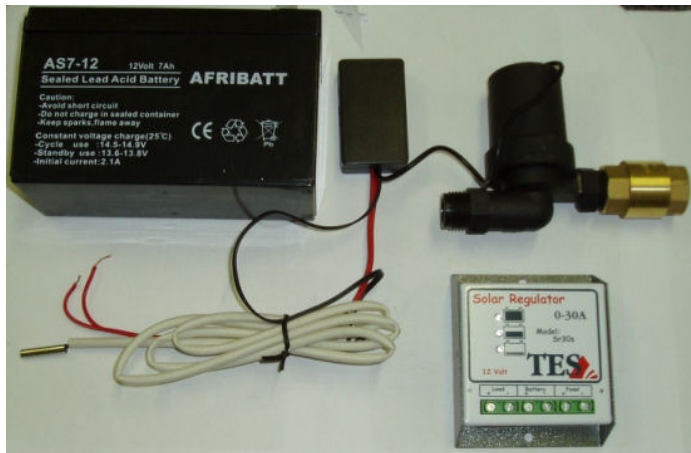
Fig 1. Pump with non return valve connected, 1Sense controller, charge controller and battery
